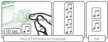
**Attention** : This operation deletes all TAGs, pin codes (keypad escutcheon) or authentication fingerprint escutcheon NOTE: it does not erase the fingerprints stored in it), and enables the service TAGs
